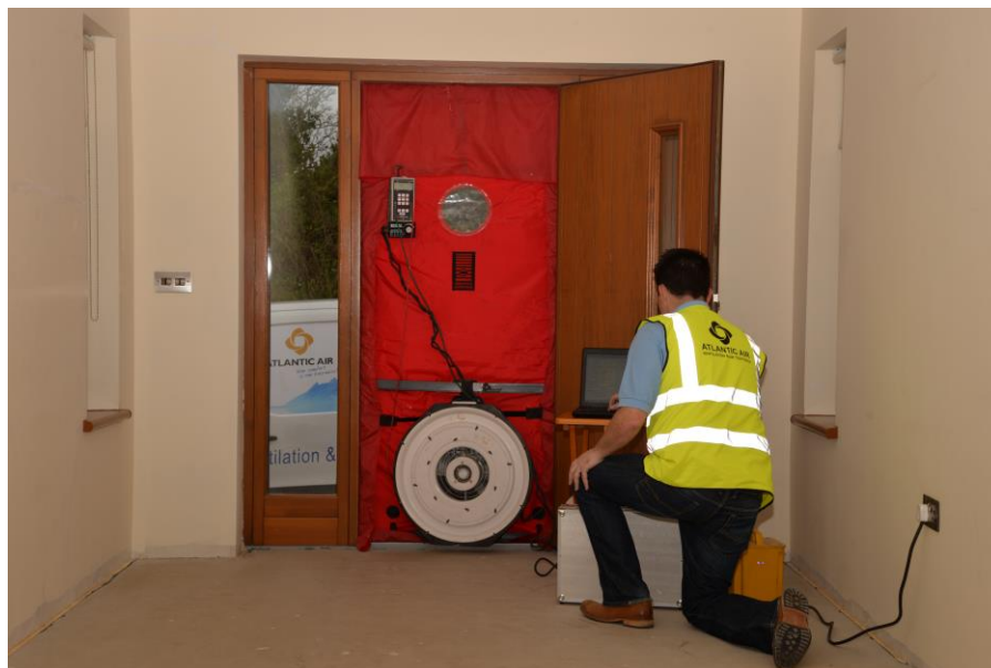
Figure 2: Air Tightness Testing on site to comply with Building Regulations
