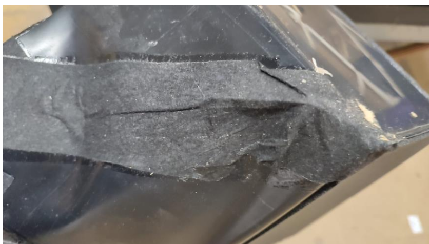
Fig.6 Uneven substrate makes attaching airtight joint tape to the corner difficult (sample #1)
